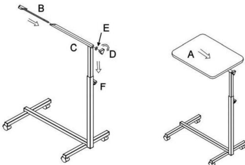
Slide the table top A into the sliding tube C and tighten the clamping knob D.
